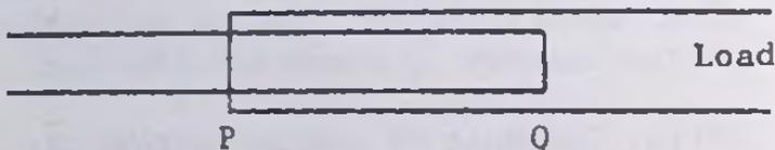
We have a complex multiple reflection situation at P and at Q and at Load. Clearly, a low (say a short) at Load will send back reflections finally calling for more input, only after alteration at Q and at P. The story is the same if primary and/or secondary have more than one turn.
